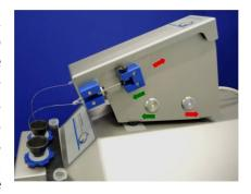
the screw of the syringe plunger pointing towards the side to avoid damaging the syringe and the TIP2k. Of note, when using 500- $\mu L$  microsyringe tighten also the front screw in TIP2k series A or B.
