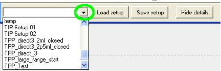
After a new setup was selected the Load setup button will be highlighted in <a href="yellow">yellow</a>. Clicking on Load setup will then load the new Setup into the TIP control window. Any unsaved changes to the current Setup will be lost. The Load setup and Save setup buttons are available from all tabs of the TIP window.
