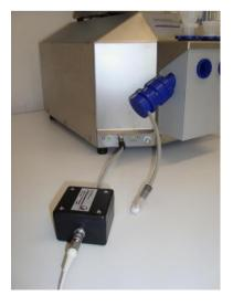
Connect the NO sensor to the NO amplification box. The NO sensor is then inserted into the other chamber that is still
