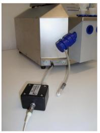
Connect the NO sensor to the NO amplification box. The NO sensor is then inserted into the other chamber that is still
