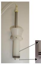
Insert the NO sensor into the stopper with the 2.3 mm additional port. Fix its vertical position by applying a small O-ring on the shaft of the NO sensor (O-rings from old NO sensor sleeves are suitable). The NO sensor should protrude from the stopper by only a few millimetres, low enough to be in a well-stirred zone but high enough not to interfere with the stirrer.
