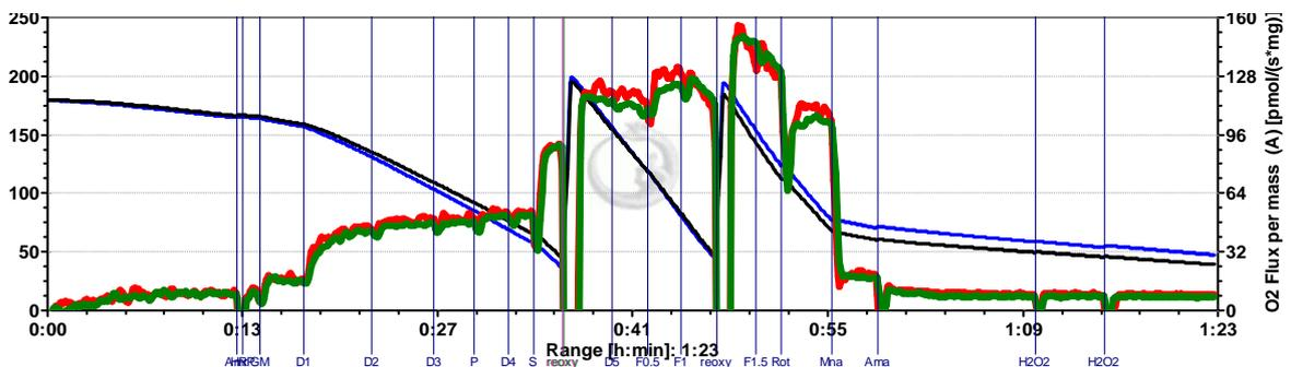
**Fig. 7:** Overlay of O<sub>2</sub>k-trace of chamber A and chamber B. Oxygen concentration [μM] (black and blue line) and oxygen flux per mass [pmol·s<sup>-1</sup>·mg<sup>-1</sup>] (red and green line) of mouse liver homogenate in MiR05.
