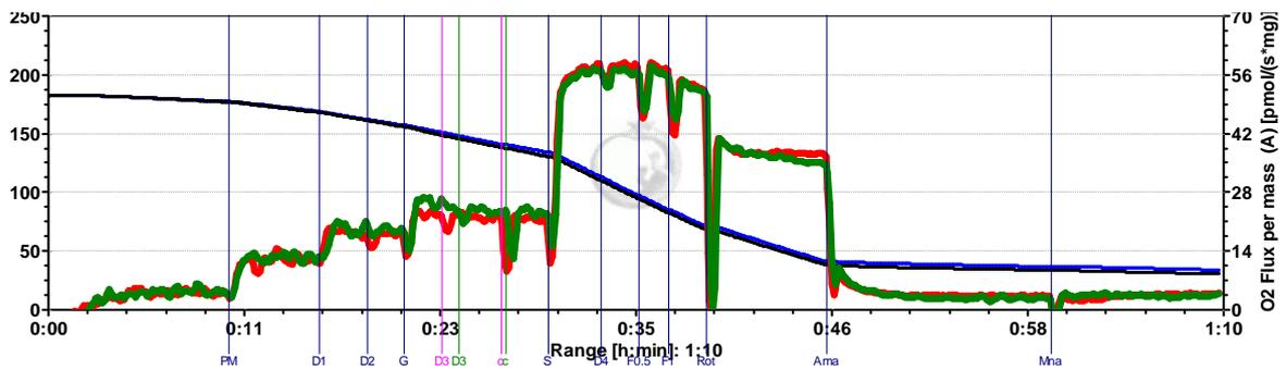
**Fig. 4:** Overlay of O<sub>2</sub>k-trace of chamber A and chamber B. Oxygen concentration [μM] (black and blue line) and oxygen flux per mass [pmol·s<sup>-1</sup>·mg<sup>-1</sup>] (red and green line) of mouse brain (cortex) homogenate in MiR05.
