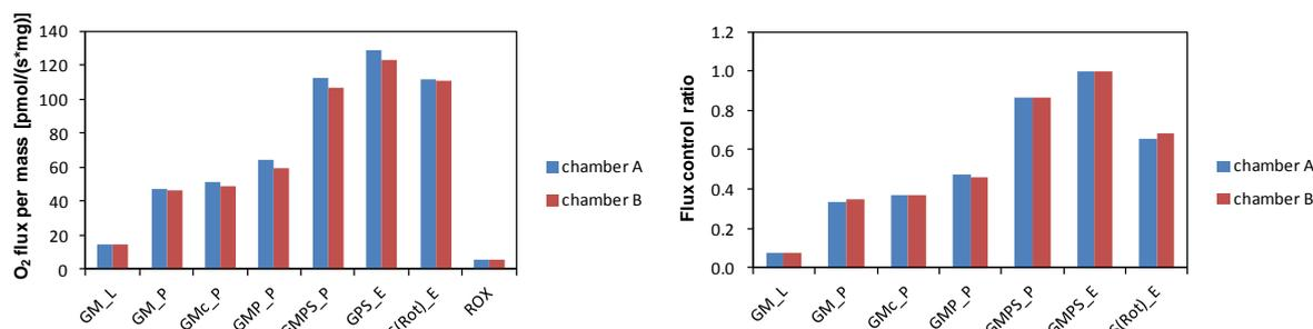
**Fig. 8:** O<sub>2</sub> flux per mass [pmol·s<sup>-1</sup>·mg<sup>-1</sup>] and flux control ratio normalized to PMGS<sub>E</sub> and corrected for ROX, of chamber A and chamber B, in mouse liver homogenate.
