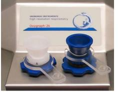
We recommend to replace titanium stoppers with the new PEEK stoppers and corresponding O2k-Chamber holders.
