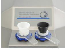
**Stopper-spacers** used for air calibration with white PVDF stopper (Chamber A) or black PEEK stopper (Chamber B). addition of the medium.
