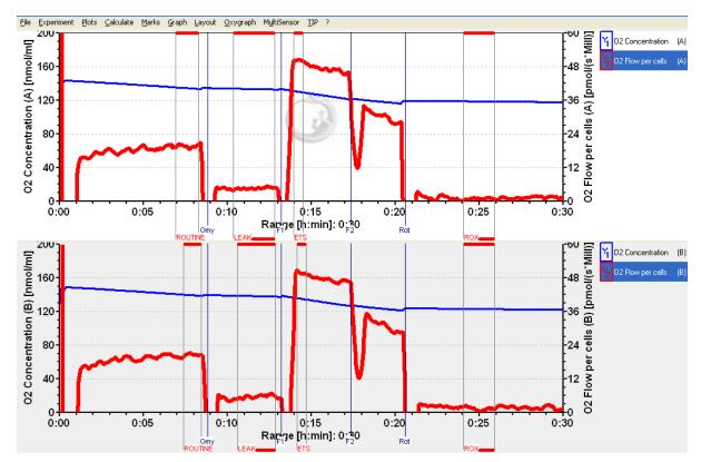
**MiPNet08.09\_2003-03-29 P1-02\_Cells.DLD**  $O_2$  concentration (blue,  $Y_1$  axis) and  $O_2$  flux (red,  $Y_2$  axis) as a function of time. Data recording was started (Connect [F7]) after adding a cell suspension at a density of  $1\cdot10^6$  cells/ml. Events are shown by vertical lines, with the <Event name> below. Marks are shown by horizontal bars between two vertical lines, with the Mark name in the lower bar.
