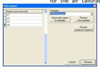
steps of oxygen concentration, the oxygen consumption by the sensor decreases linearly, and the effect of oxygen backdiffusion is finally apparent as a positive slope or negative flux (Marks Jo to Jo 4). Mark names are selected from the pull down menu Graph \ Names, selecting the template "O2kBackground".
