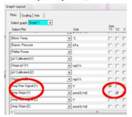
based on the recorded signal: Amp Raw Signal, Amp Calibrated, and Amp Slope. These plots can be selected from the drop-down lines and displayed with their check boxes either on the Y1 or the Y2 axis [Graph layout / Select Plots].
