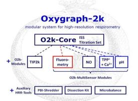
The O2k-Fluorescence LED2-Module is a modular extension of the O2k-Core (Series D-F). A growing number of fluorescence markers enables determination of diverse mitochondrial addition processes in to oxygen consumption, including generation of production, mitochondrial  $H_2O_2$ , ATP potential  $Ca^{2+}$ membrane and extendable by user-specific applications.
