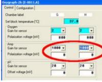
Fluo-Sensor (O2k-Chamber A and B) is controlled in the DatLab Control window in the field "Amp Polarisation voltage [mV]" (0 to 2000). Click Connect to Oxygraph-2k or Send to Oxygraph to apply the new settings.
