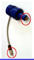
Within the stainless steel Oxygraph-2k housing, internal electronic components are well protected from ESD. However, during chamber assembly, membrane change, or trouble shouting, the polarographic oxygen sensor (POS) has to be disconnected from the POS connector and the POS connector is disconnected from the main unit. This means that one or both electric connections of the POS connector are exposed to the environment and ESD damage is possible.
